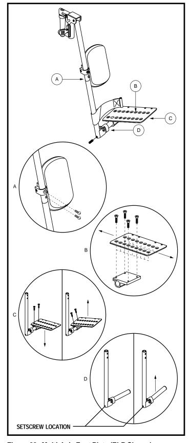
Figure 23. Multi-Axis Foot Plate (ELR Shown)
